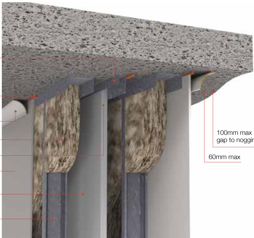
FIGURE 36 – SECTION OF STEEL FRAME SLAB TO SLAB PARTY WALL SYSTEM
